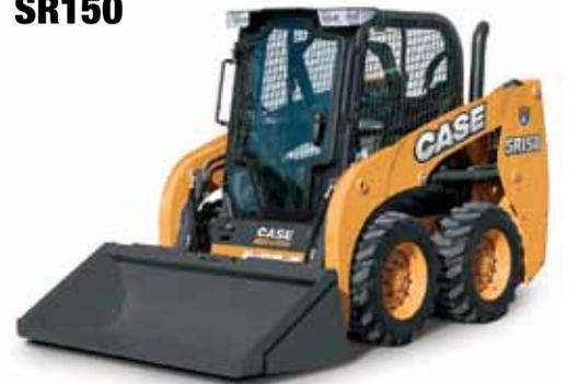
The Case SR130 and SR150 skid steers offer rated operating capacities (ROC) of 1,300 and 1,500 lb (590 and 680 kg), respectively. Easy to transport with a trailer, both models have an extremely low overall height, at 75 in (1900 mm), making it easier to clear overhead obstacles.
