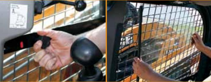
Standard features include an interior dome light and three-piece side windows that can be removed in seconds without tools.
