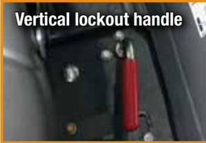
Loader lock devices and hydraulic pressure release valves create better maintenance conditions.
