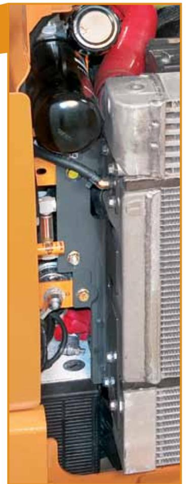
Other standard service-related features include a master disconnect switch, sight gauge and easy-access filters.
