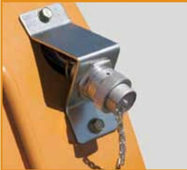
A 14-pin Front Electric system provides four independent activation systems that can be called up with the touch of a button on the control handles.
