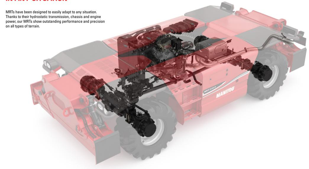
Hydrostatic transmission ensures maneuverability and ease of use.
