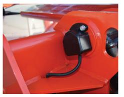
MRT 2470 and 3050 models sit on stabilisers equipped with strain gauges for greater precision in all surfaces.
